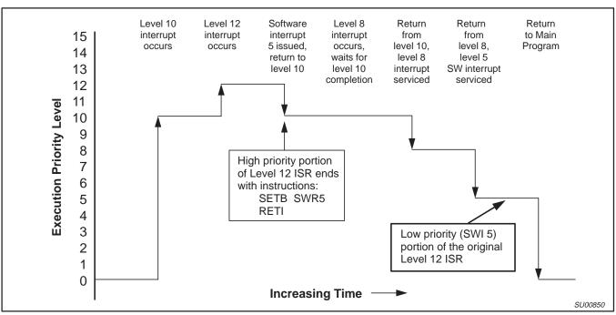
Figure 3. Correct Priority Execution with Software Interrupts
