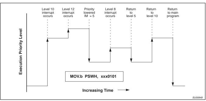
Figure 2. Priority Inversion (No Software Interrupts)
